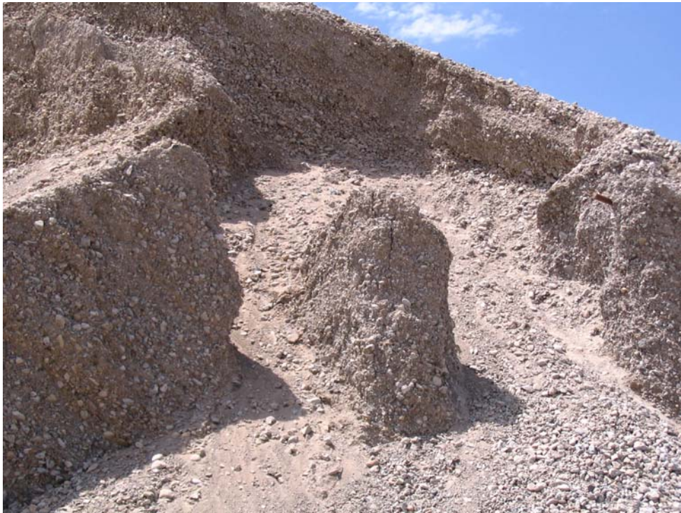
Figure 4.29. Segregation of stockpiled RCA at Mountain Home AFB.
