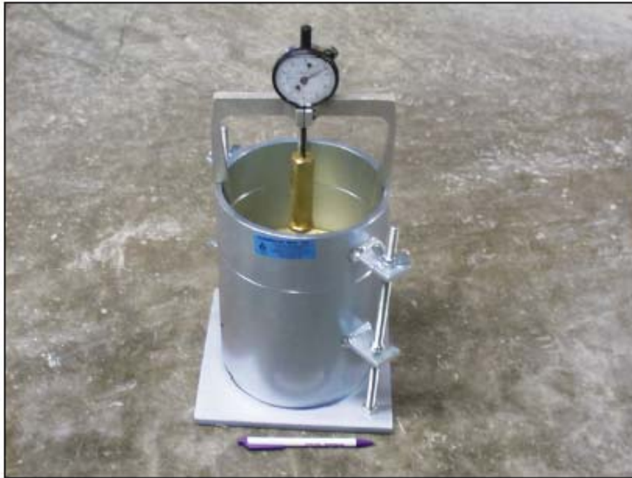
Figure A.31. Apparatus used by Rathje et al. (2002) to evaluate ASR-related expansion.
