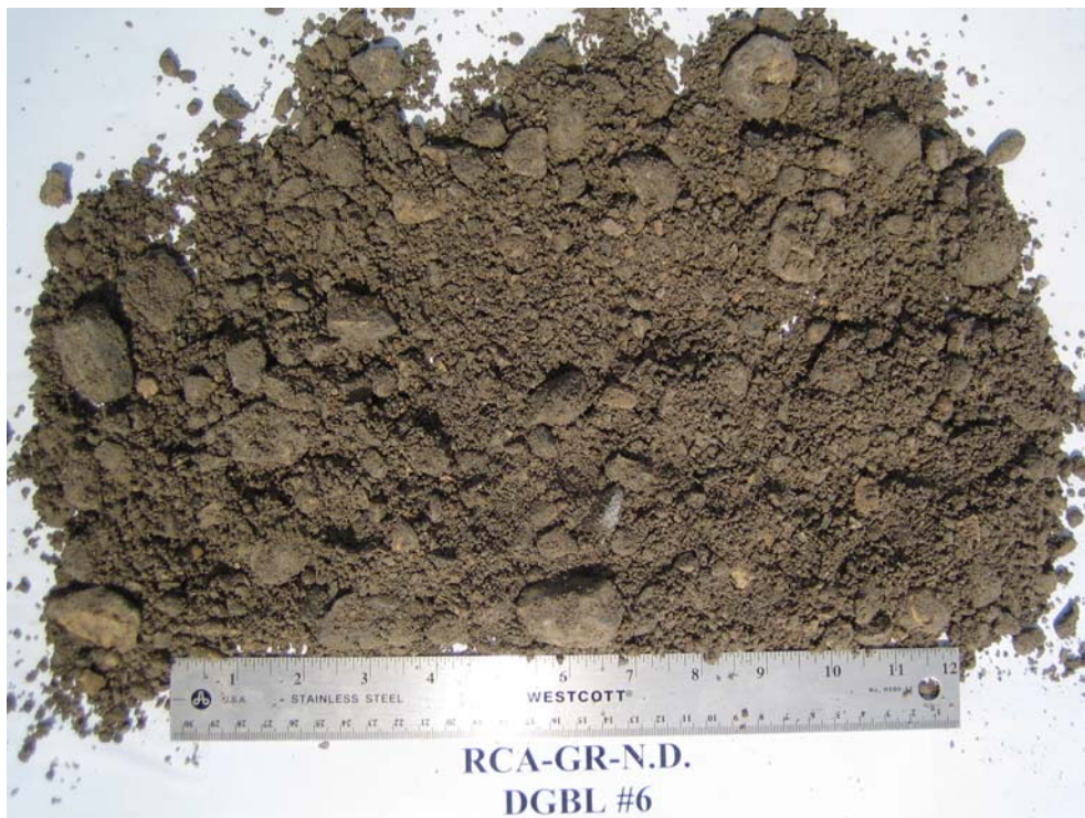
Figure 4.39. RCA material as-received from Grand Forks AFB, ND.
