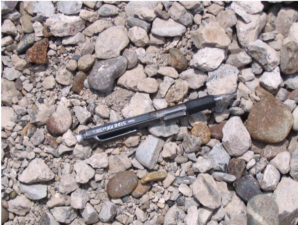
Figure 4.27. PCC at Mountain Home AFB was crushed to minus 2-inch size.
