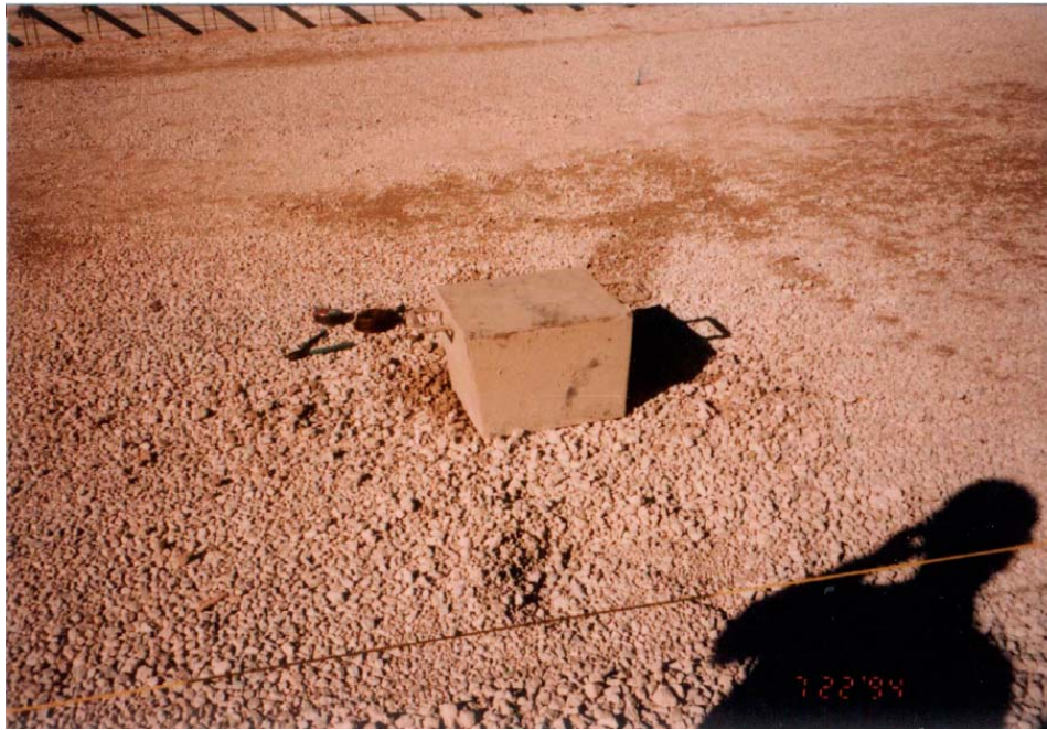
Figure 4.33. View of the compacted RCA rapid draining material.
